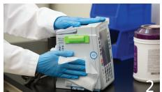
Make sure the instrument is upright, turned off, and the power cord is unplugged. Wipe all exposed device surfaces.
