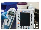
Let the IUI connectors air dry for about 15 minutes before connecting the device to another device.
