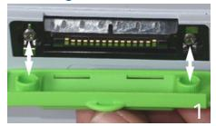
Attach IUI connector covers by aligning the round openings on the inside of the covers with the screws on the IUI connector. Ensure the tab is pointed upward when attached.
