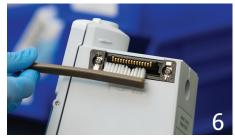
Clean both IUIs with the dedicated IUI cleaning brush. Brush the IUI connectors up and down. Do not brush them side to side as this can damage the pins.
